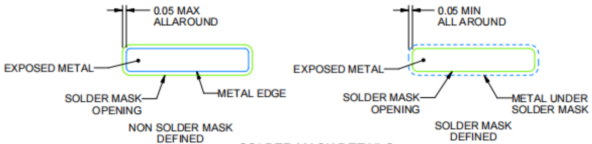
LAND PATTERN EXAMPLE EXPOSED METAL SHOWN SCALE 10.000
